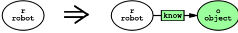
Fig. 3. Example of a graph transformation rule used to make the robot find new objects.
